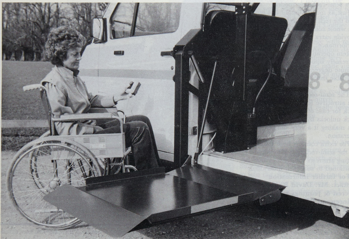
HBC 200 Automatic Wheelchair lift easily controlled from a wheelchair
