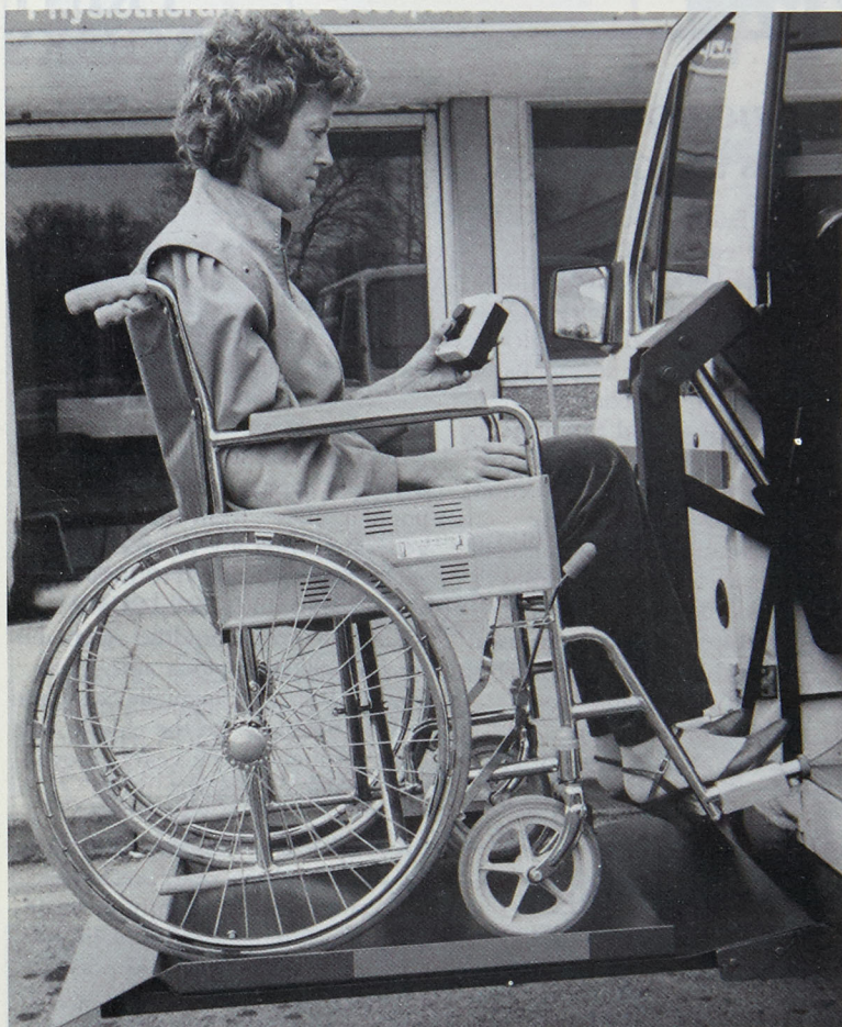
HBC 200 Automatic Wheelchair lift fully powered opening and closing. No physical effort required
